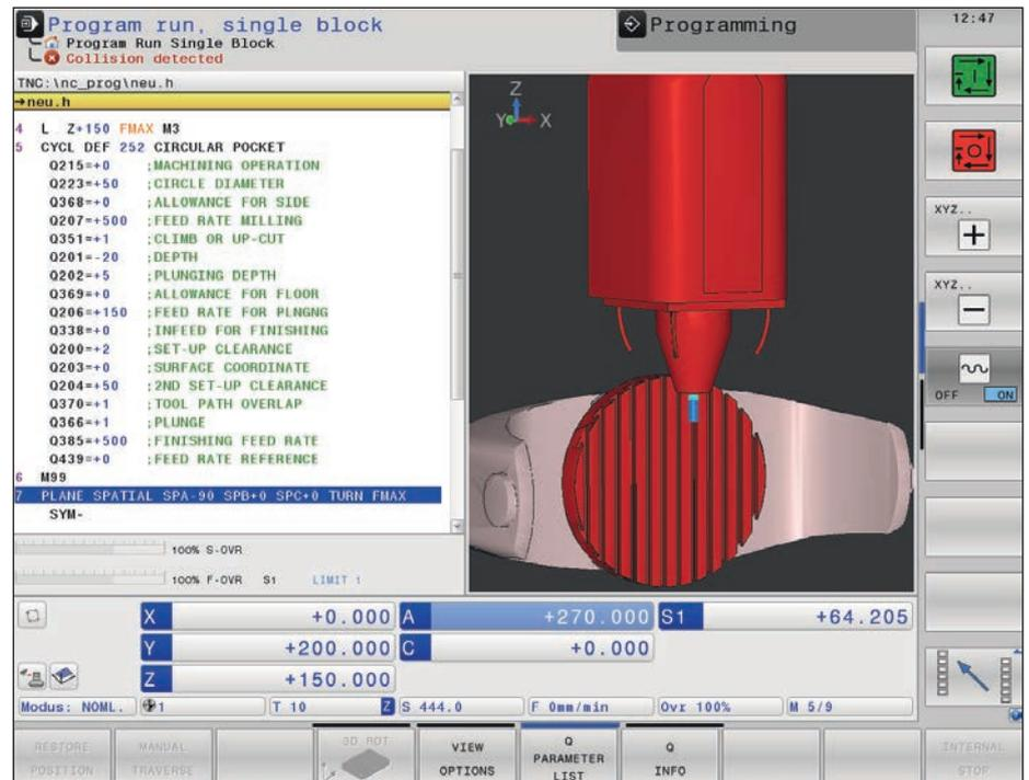
Of course, the TNC 640 also shows the operator which machine components are on a path toward collision, both in the error message and in a graphical depiction. If a collision warning is displayed, then the TNC 640 permits retraction of the tool only in directions that will increase the clearance between the colliding objects.
