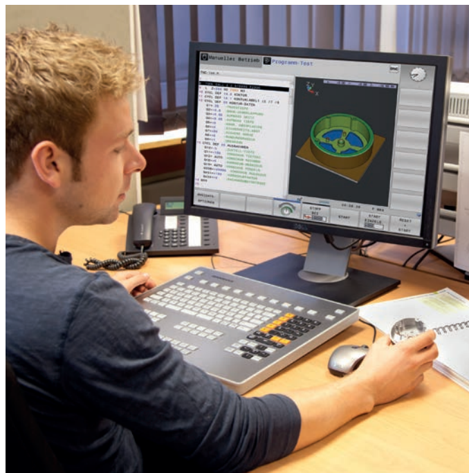
Programming station with TNC operating panel
