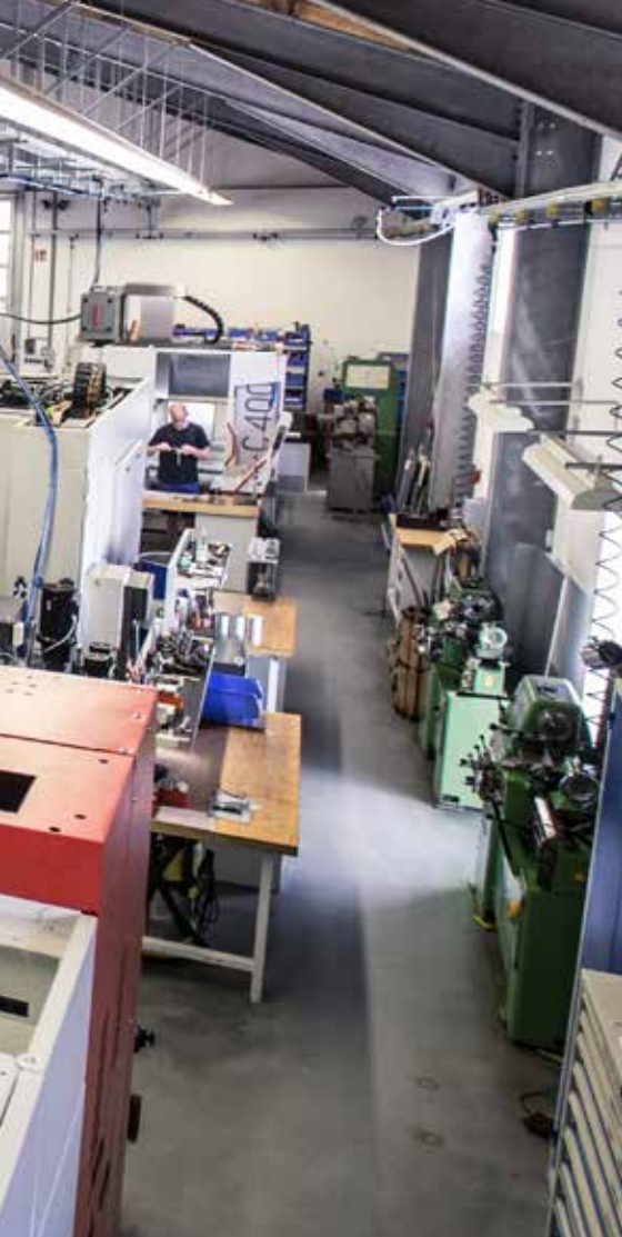
The production floor at WB mechanics: six milling machines with HEIDENHAIN controls, along with six lathes, are all connected to StateMonitor.
