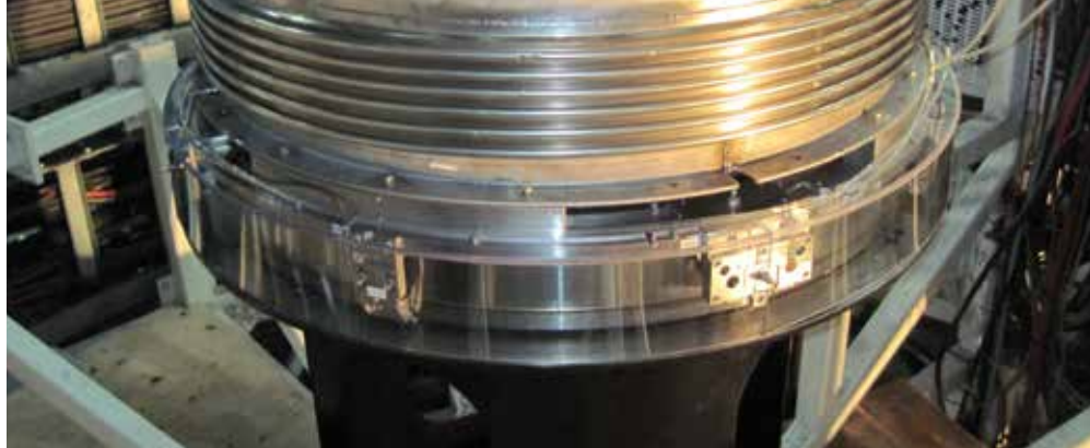
Mounting configuration of the ERA 8400 angle encoders on the telescope drive system for azimuth positioning
