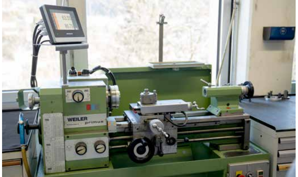
Altogether, eight conventional, manually operated machines were converted as part of the retrofit.
