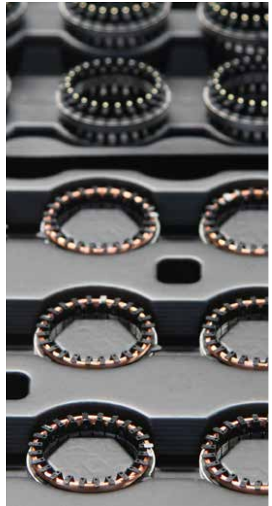
Before and after: Finished stator winding cores below and empty ones above.
