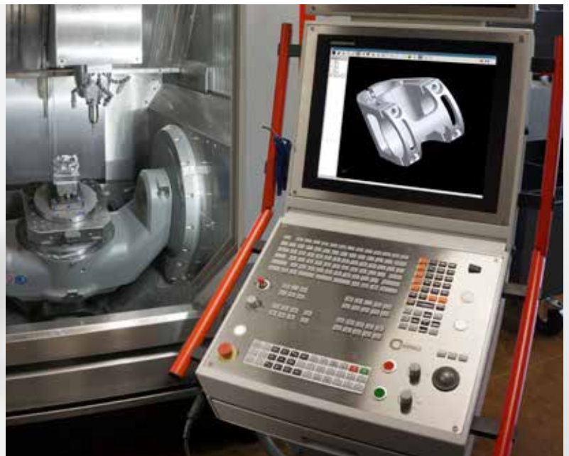
The 3-D data of a complex component, like this mountain bike handlebar mount (above), can be loaded directly into the NC program.
