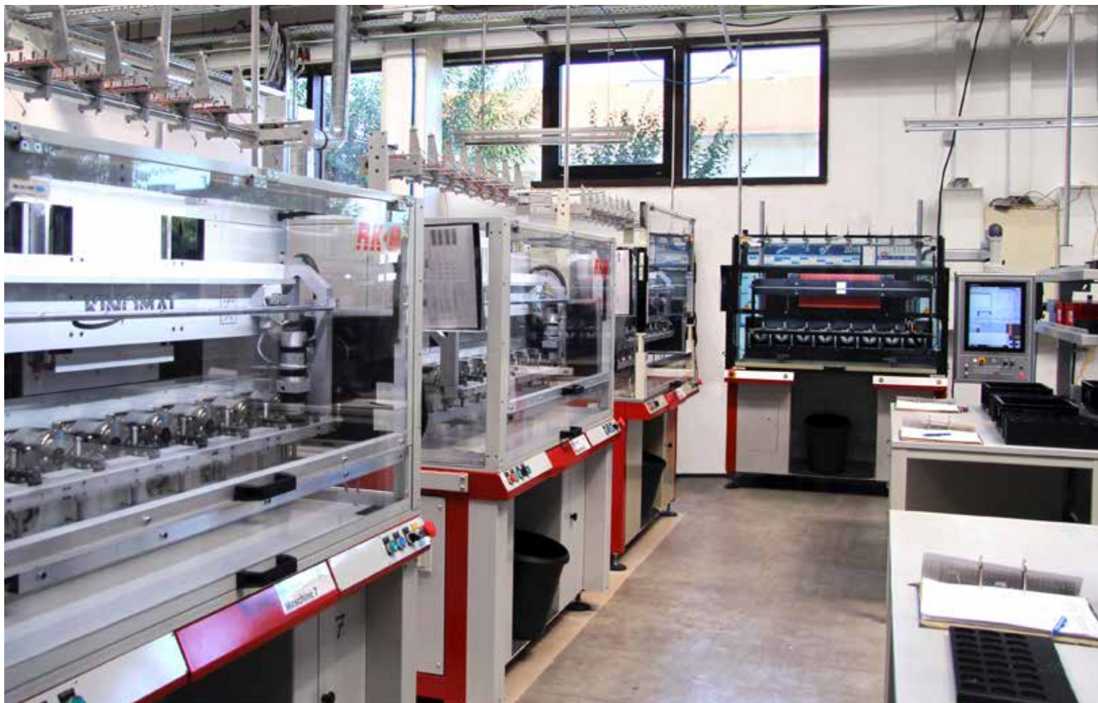
The upgraded resolver winding machine with TNC 620 control is located at the head end, with three of the six systems to be retrofitted by the end of 2019 on the left.
