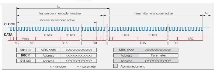
Typical EnDat 2.2 command sequence for transmitting a position value with parameter values in the additional information (max. 12 ms access time by interrogating the integrated EEPROM)
