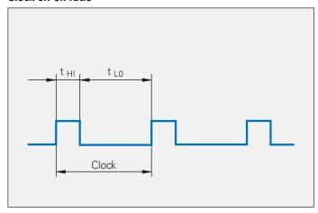
between the last rising clock pulse edge and the edge of the start bit. The process should be repeated at least three times in order to rule out any disturbances during the calculation of the propagation time and to test the value for consistency. The signal propagation time is measured at a reduced clock frequency (100 kHz to 200 kHz). To attain sufficient accuracy, however, the
