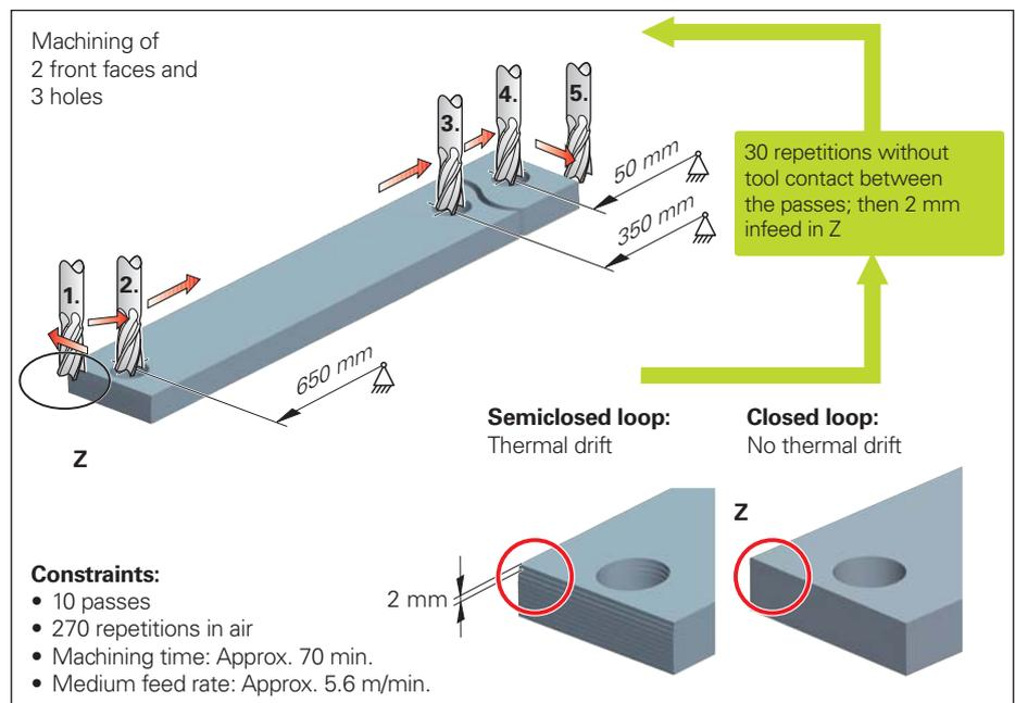
Figure 4 Effect of drive accuracy on series production
