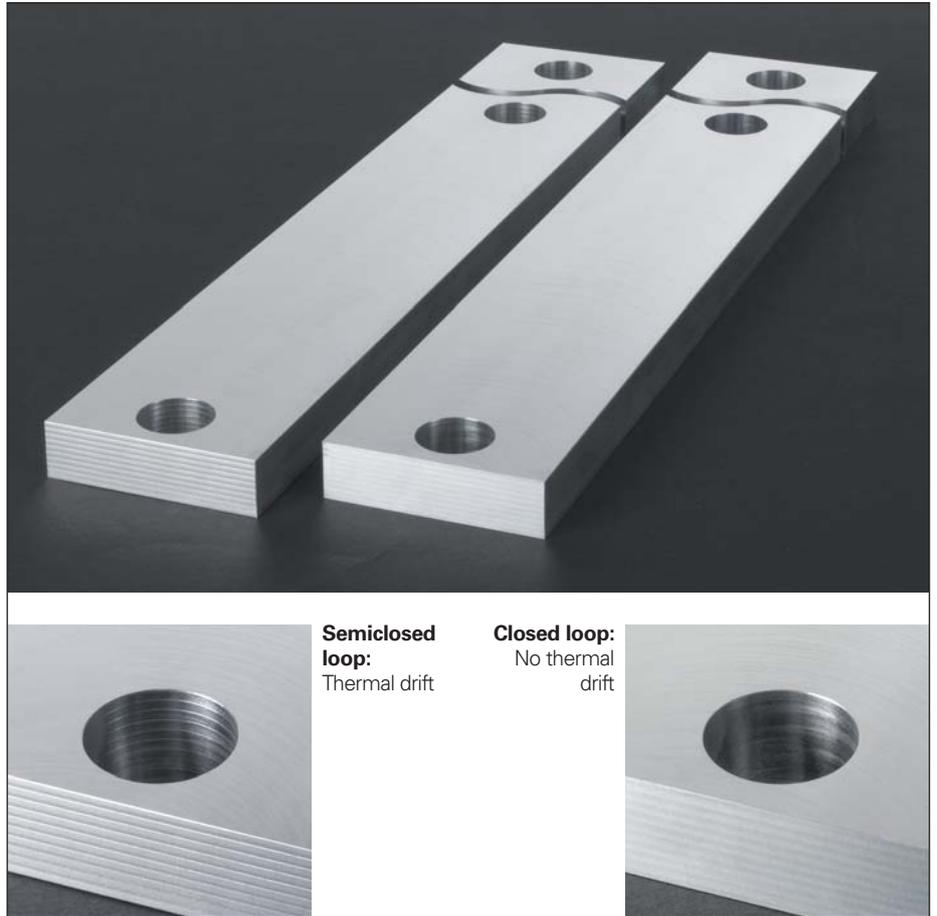
Figure 5 Deviation between hole patterns in series production
