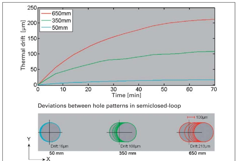
Figure 6 Drift at various positions in the traverse range of the X axis (ISO 230-3)
