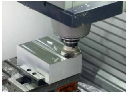
Mean power consumption of the drives during rough facing Face-milling cutter: D = 60 mm, speed: 4 100 rpm, infeed depth: 4 mm
