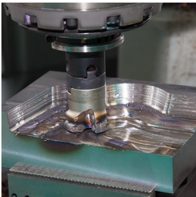
Workpiece with damage resulting from a broken indexable insert
