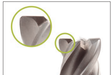
Machining with OCM: Tool after six parts
