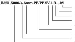
Flange fastening screws Without housing Direction of connection for PCB connector Reference mark Supply voltage Interface Shaft diameter Commutation Signal periods per revolution
