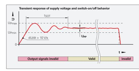
t<sub>SOT</sub> = Typical: 1.3 ms Max.: 2.6 ms
