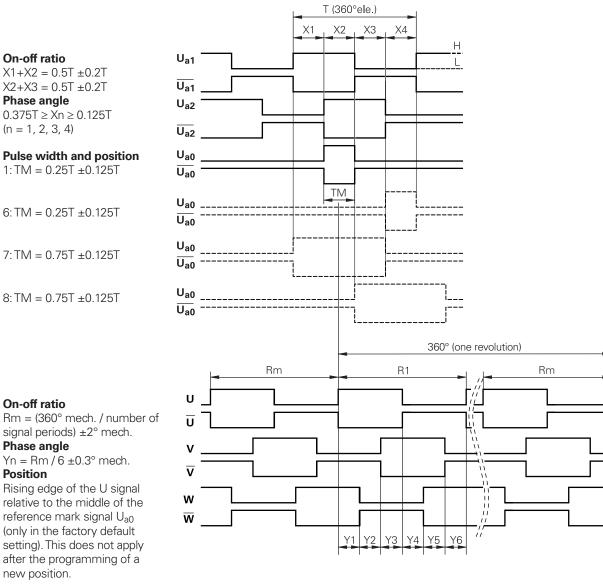
$\begin{array}{l} U_{a1}, \, \overline{U_{a1}}, \\ U_{a2}, \, \overline{U_{a2}} \end{array}$ **On-off ratio**  $X1+X2 = 0.5T \pm 0.2T$  $X2+X3 = 0.5T \pm 0.2T$ Phase angle  $0.375T \geq Xn \geq 0.125T$ (n = 1, 2, 3, 4)
