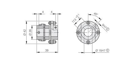
€-]⊕ Tolerancing ISO 8015 ISO 2768 - m H ≤ 6 mm: ±0.2 mm
