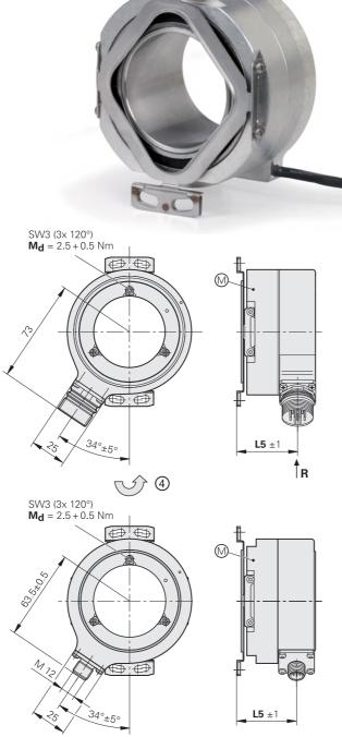
Connector coding  $\mathbf{R} = \text{Radial}$
