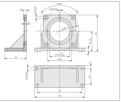
mm ----Tolerancing ISO 8015 ISO 2768 - m H ≤ 6 mm: ±0.2 mm
