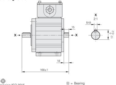
mm -----Tolerancing ISO 8015 ISO 2768 - m H < 6 mm: ±0.2 mm
