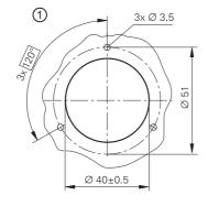
1 = Cutout for mounting2 = Direction for output signals as per the interface description
