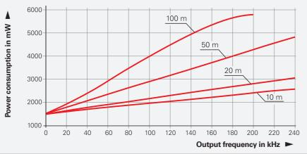
Power consumption (maximum) for the HTLs interface and supply voltage  $U_{\rm P}$  = 30 V
