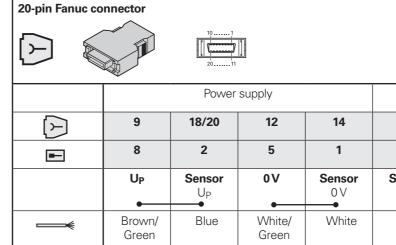
**Cable shield** connected to housing;  $U_P$  = Power supply voltage
