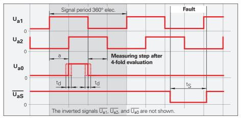
The distance between two successive edges of the incremental signals  $U_{a1}$  and  $U_{a2}$  through 1-fold, 2-fold, or 4-fold evaluation is one **measuring step**.
