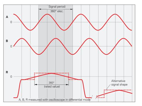
HEIDENHAIN encoders with the TLITTL interface incorporate electronics that digitize sinusoidal scanning signals with or without interpolation.
