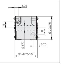
\* With typical mounting tolerances: radial offset  $\lambda = 0.1$  mm; angular error  $\alpha = 0.09^{\circ}$  (0.15 mm over 100 mm)
