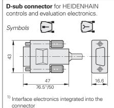
The **pin numbering** on connectors is in the direction opposite to that on couplings or flange sockets, regardless of whether the connecting elements have
