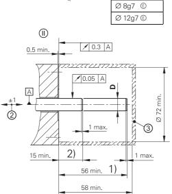
mm  $\Box$ Tolerancing ISO 8015 ISO 2768 - m H < 6 mm: ±0.2 mm
