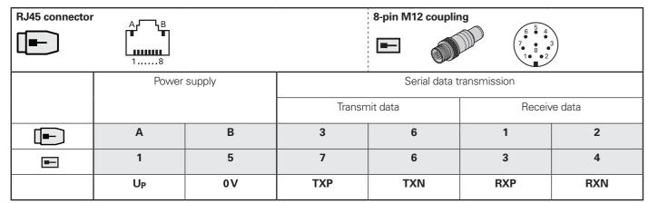
**Cable shield** connected to housing;  $U_P$  = Power supply voltage
