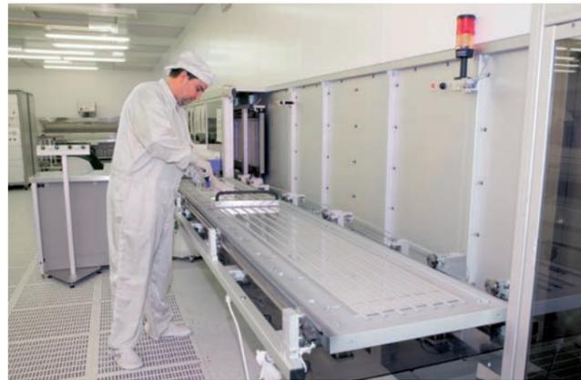
Vacuum machine for application of chromium layers
