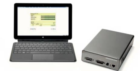
PWM 21 inspection device with included ATS adjusting and testing software
