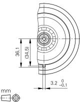
Tolerancing ISO 8015 ISO 2768 - m H < 6 mm: ±0.2 mm
