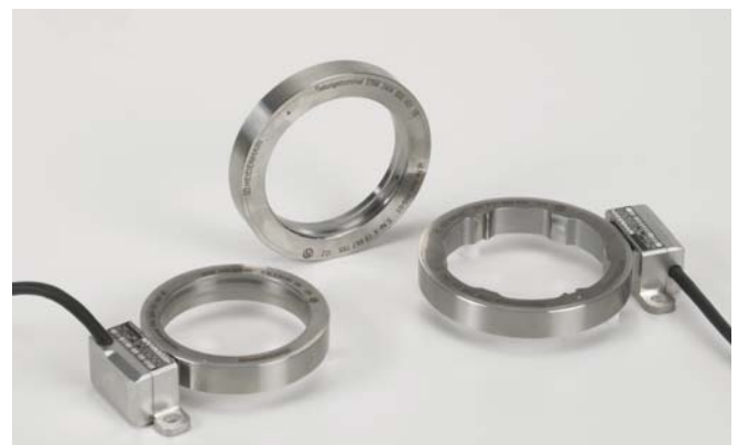
2: The ERM 2400 series encoders consist of a scanning head and a circumferential-scale drum. The latter is available with smooth inside contour or with a keyway as anti-rotation element.
