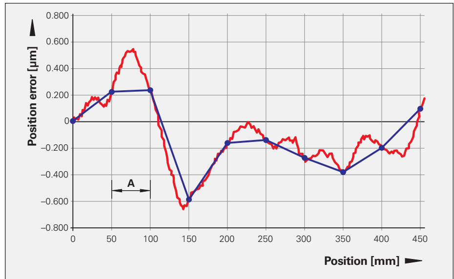
Figure 2: Compensation points for multipoint linear error compensation
