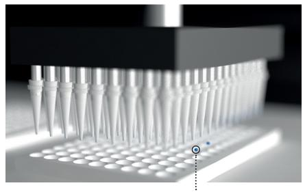
Spilling may occur when a conventional system is sped up to achieve higher throughput. Vibrations are introduced in such drives, which support spilling of small droplets. With technologies from ETEL and HEIDENHAIN the motion of the instrument is fast and very smooth at the same time. Vibrations are at a very low level and consequently contamination of the instrument by spilling is avoided.
