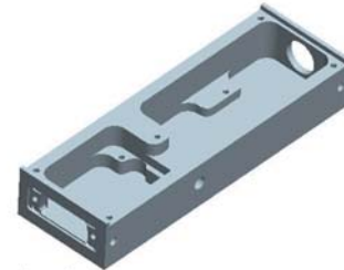
Housing for the observation of the power requirements of a milling process
