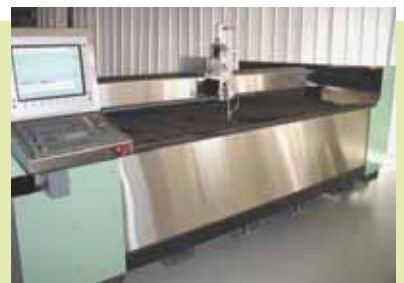
Stone Contour Systems' Contourjet 510 with HEIDENHAIN's iTNC 530 control and scales, and ETEL's linear motor.
