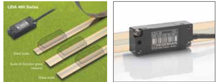
The scanning heads for the LIDA 400 are a standard size, so they meet all requirements for reading the scales of glass and glass ceramic. Also, the identical cross section of the scales allows the graduation carriers to be exchanged.
