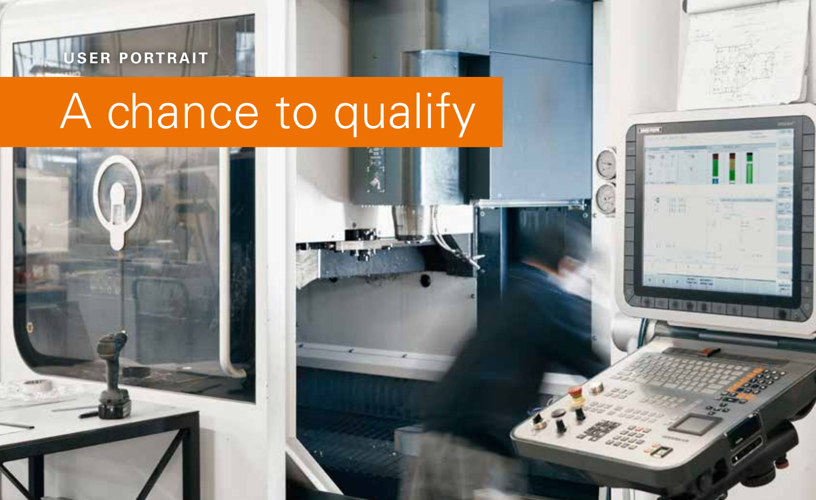
Among other production equipment, the shop features two DMG milling machines with HEIDENHAIN iTNC 530 controls for training purposes.
