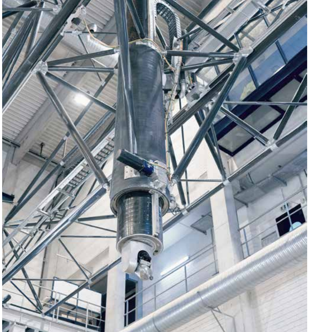
This completely revamped portal machines the lower workpiece heights of approximately 1 m to 4 m.
