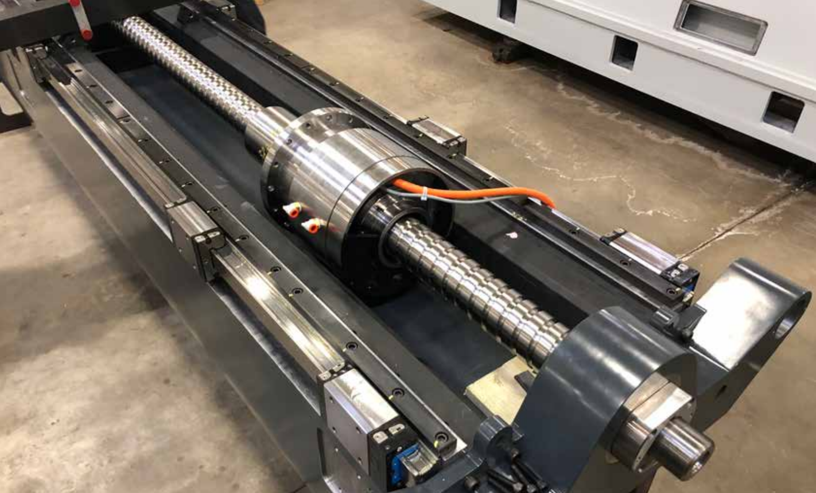
ETEL torque motor-equipped direct drive ball-nut assembly at TARUS.
