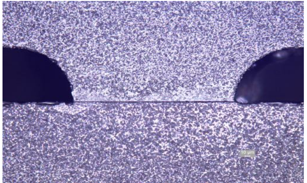
UV Adhesives room temperature glass:glass bond used to preserve bioactivity of encapsulated biomolecules/cells. A >0.3mm glass wafer with isotropically etched channels bonded with UV-adhesive to a 1mm thick glass wafer. (Source: IMT)
