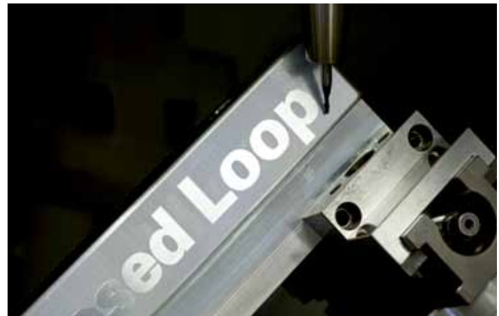
Semi-closed loop: Accuracy-limiting influences from the drive mechanics have no influence on the results of machining. Thanks to the precise angle encoders from HEIDENHAIN, a high contour accuracy and excellent surface definition of the workpiece are achieved.
