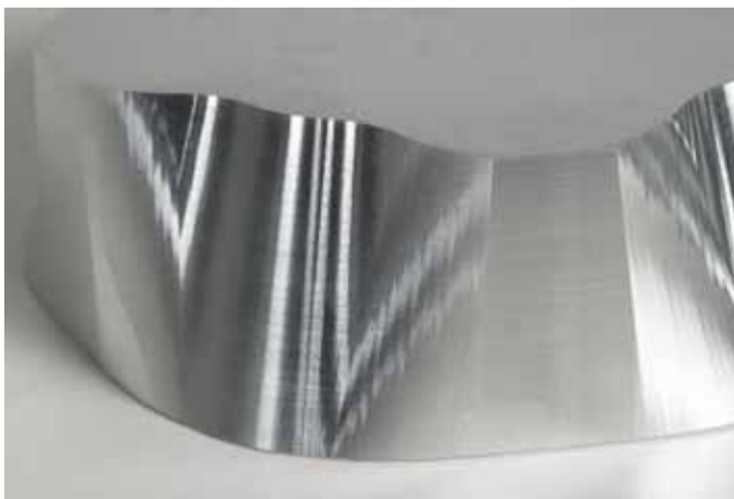
Semi-closed loop: Polygonal workpiece with surface error.
