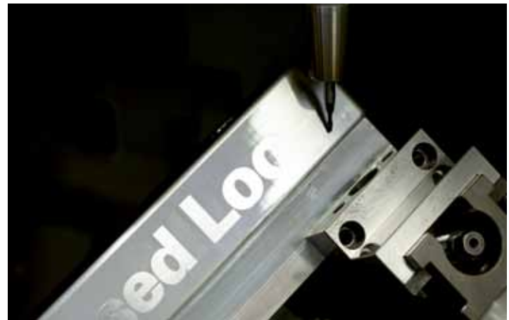
Semi-closed loop: Influences on the drive mechanism (e.g. transmission errors) can impair the machine's accuracy and therefore the machining accuracy and surface quality.
