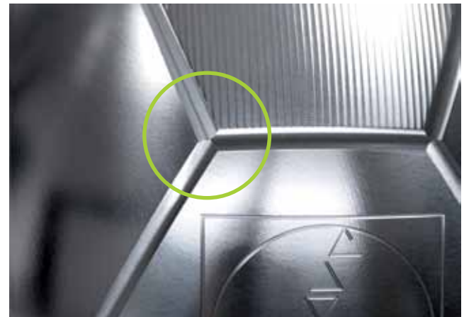
Closed loop: Thanks to the precise linear and angle encoders from HEIDENHAIN, errors in the drive mechanics have no influence on the result of machining. The seams are milled to the correct width, and the intersections all match up exactly.
