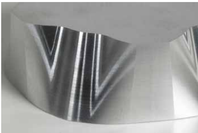
Closed loop: Polygonal workpiece with very high surface definition.
