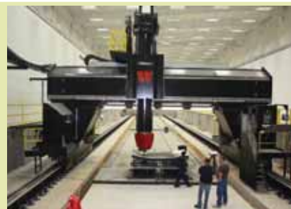
W Industries' gantry machine is 20' wide and 204' long.
